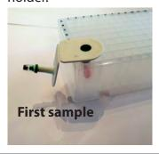
Punch a hole to remove the plastic seal.
